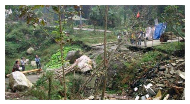
Photo 1 Examination of surface faults near hypocenter of the Wenchuan Earthquake  $({\rm Hongkou\; area})$
