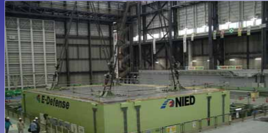
770 tonf Table (32 welded blocks) (May, 2004)
