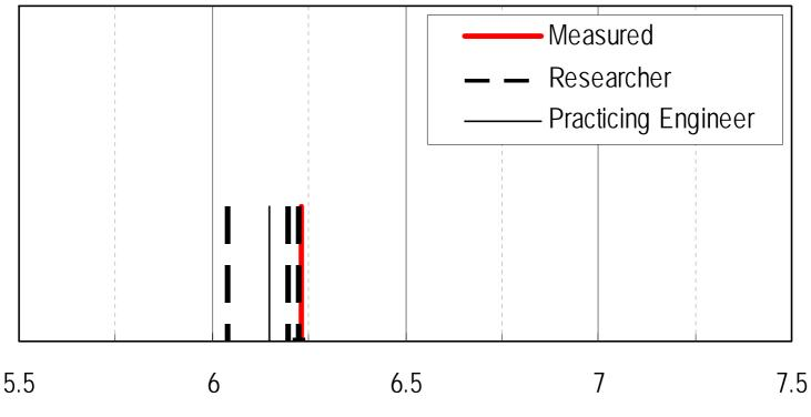
Time at which any story-drift-angle reaches 0.13 or -0.13 rad(sec) Two of the Practicing Engineers answered that any story-drift-angle didn't reach 0.13 or -0.13 rad.
