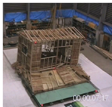
Photo 3 Preliminary 3-D shake table test on full-scale wooden frame
