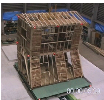
Photo 3 Preliminary 3-D shake table test on full-scale wooden frame
