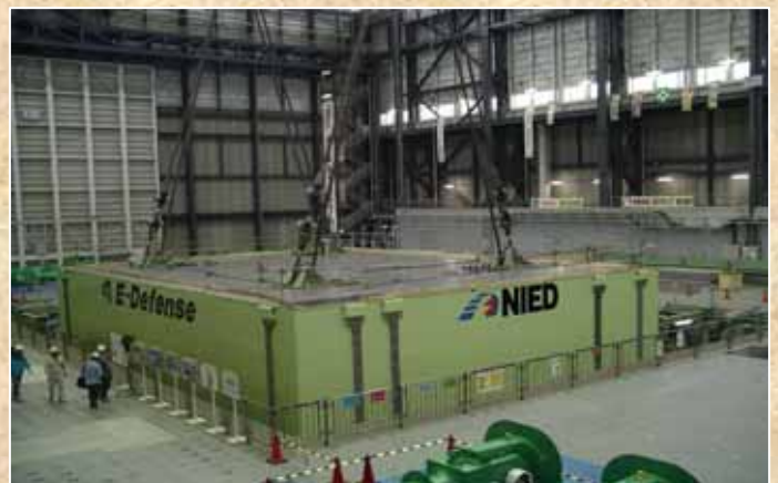
770-ton Table (32 welded blocks) (May, 2004)
