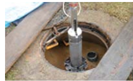
Fig. 6. Photos of fixing apparatus that utilizes the Hole lock. This apparatus is located at the top and bottom of the protective housing of a seismometer. Left panel: view of the inside; right panel: external view.
