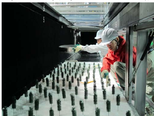
森林内の融雪特性に関する風洞実験 Wind-tunnel experiment on the effects of forests on snowmelt.
