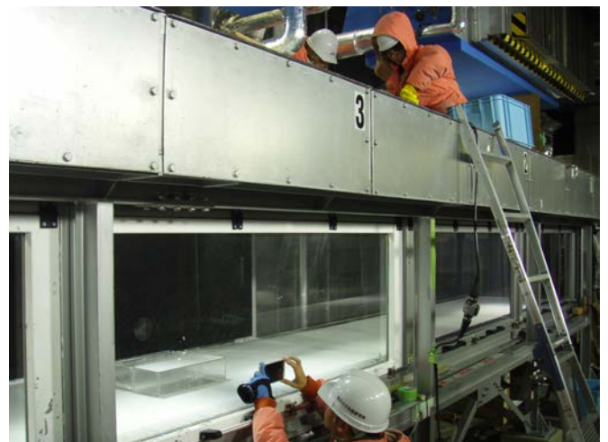
風洞装置を用いた模型屋根への雪の堆積実験 Experiment of snow accumulation on a model of roofs using the wind-tunnel.
