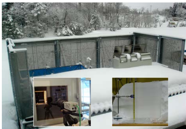
防風ネットを備えた降雪粒子観測施設 Falling Snow Observatory surrounded by the wind shielding net.
